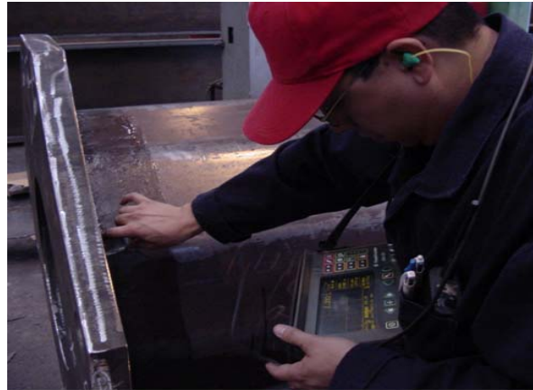
Fig . 10 : UT Inspection of Base plate Weld
