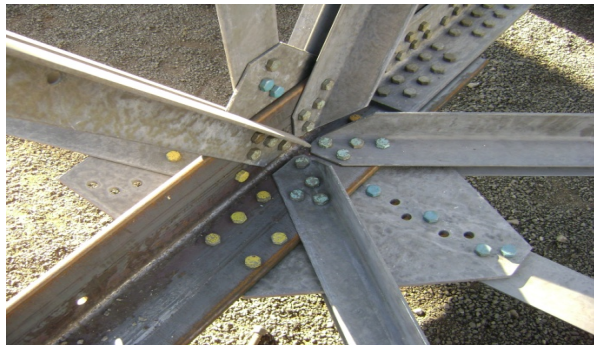
Fig. 26: Proof-of-fit of tower connection
