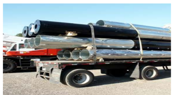
Fig . 19: Pole sections on truck.
