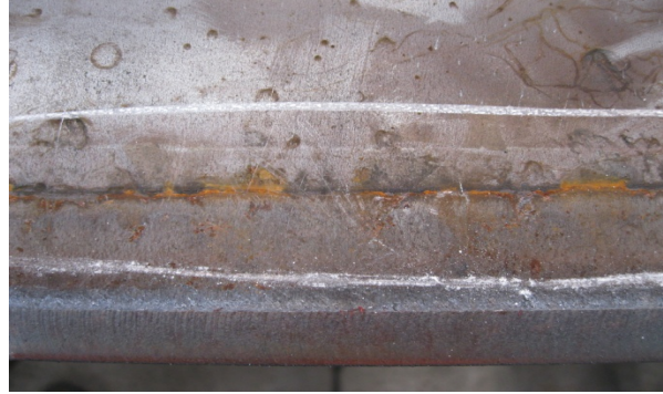
Fig. 23: Surface flaw found on steel profile
