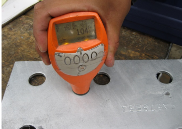
Fig.28: Measuring thickness of galvanizing
