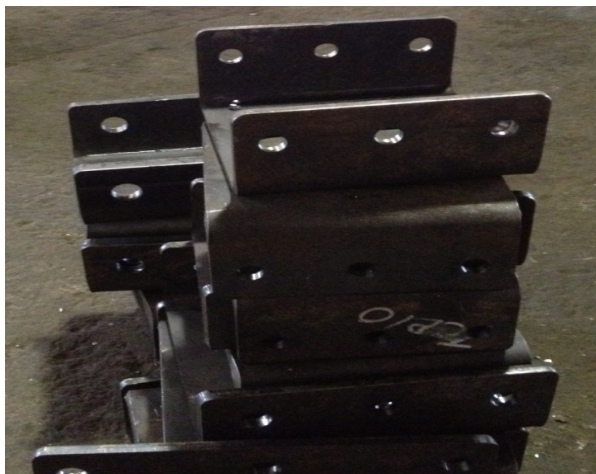
Fig . 13: Inspection of arm brackets
