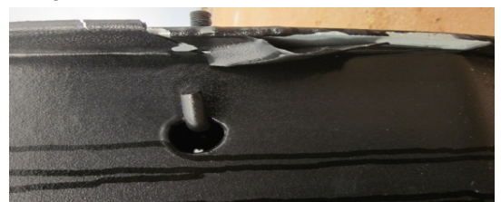
Fig . 20: Coating damage during shipment
