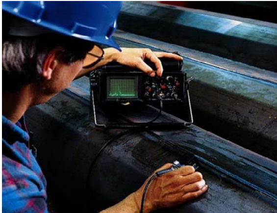
Fig . 9 : UT Inspection of Seam Weld
